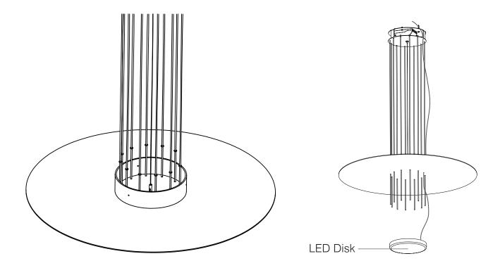
5. Raise the diffuser plate and thread the rods through the holes on the plate, then thread the power cable of the LED disk through the diffuser plate and through the canopy disk.
