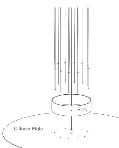
4. Pass the steel wire through the ring and insert the wire through the cable gripper. Adjust the length of the steel wire to adjust the height of the diffuser plate as desired.
